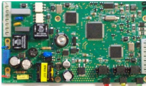
Figure 8: charging spot electronic board (74mm x 135 mm)
